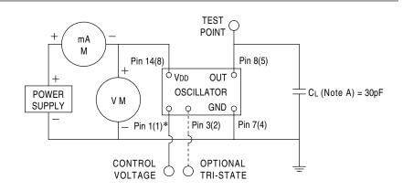
NOTE A: C<sub>L</sub> includes probe and fixture capacitance \* Items in brackets() represent Half Size model
